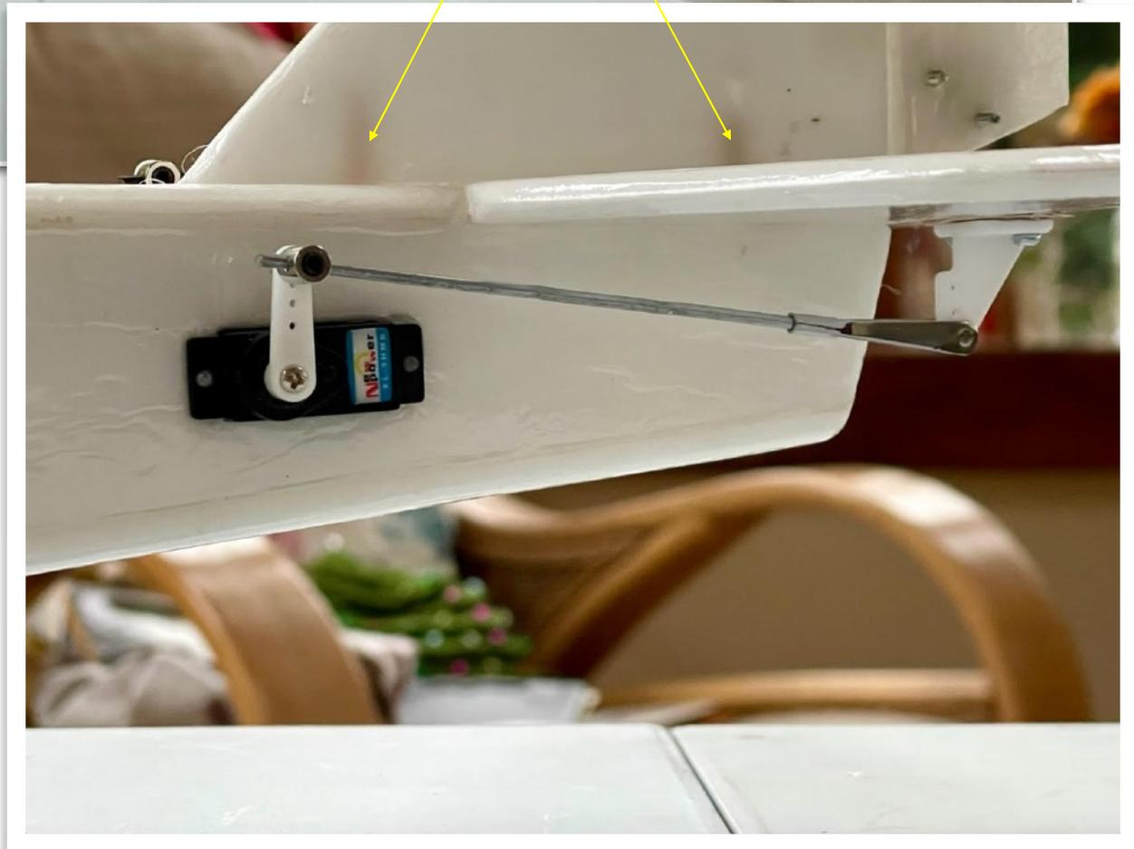
The aileron servos were fitted by simply cutting out holes in the wings and holding the servos in place with clear packing tape!
