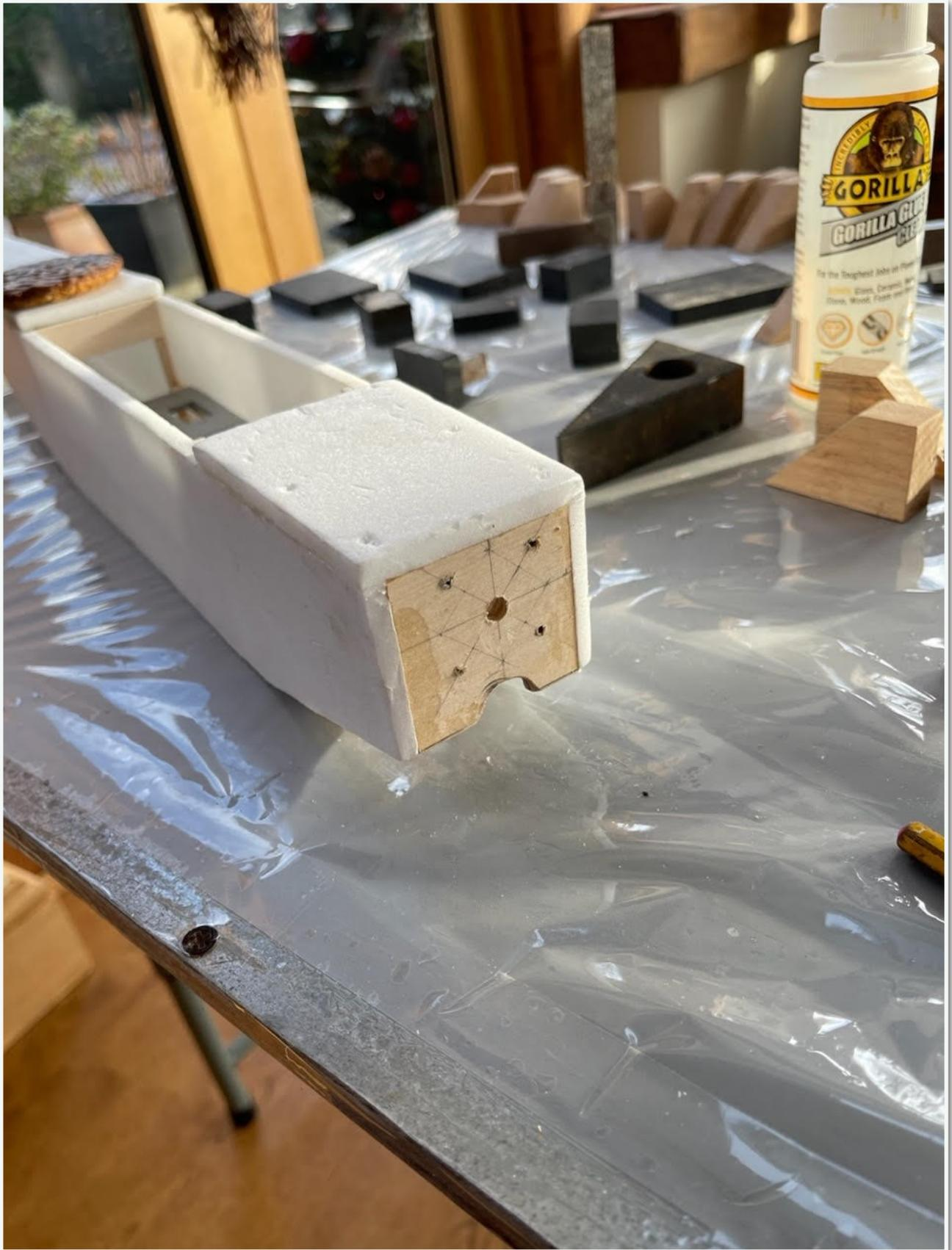
Underside nose and belly sheeting was then added to complete the fuselage 'box'.
