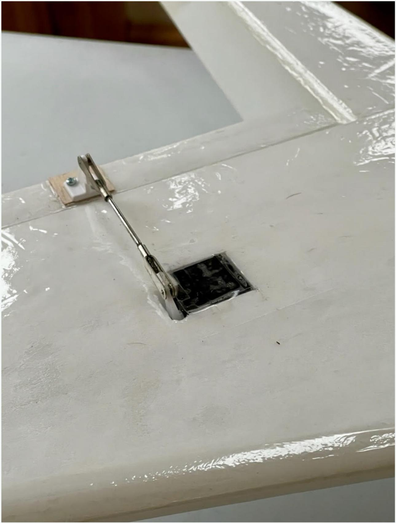
Finally the under fuselage battery access hatch was hinged using reinforced tape and a latch made from an old servo horn.
