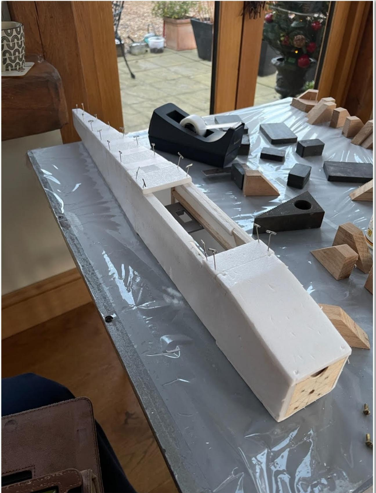
The great thing about Depron is how easy it is to sand so an hour later all components have been rounded or aerofoil sections created which then meant that I could apply laminating film. This works great on a lower than normal (100°) setting and doesn't damage the foam, but is optional.
