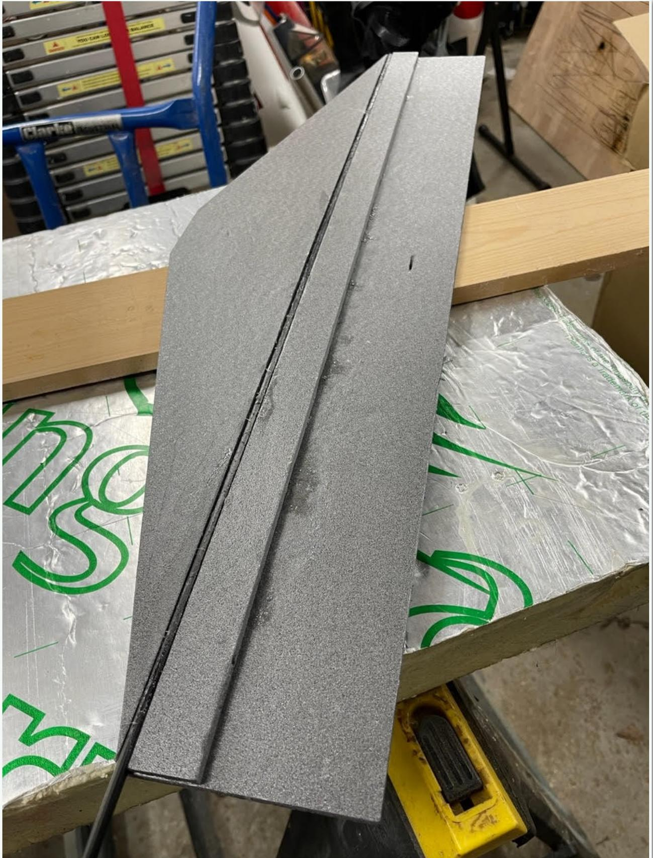
It's loosely based on the KfM-2 aerofoil which has the step at 50% chord. Not sure how that relates to a swept LE wing like the Hanky Planky so will be interesting to see how it performs.
