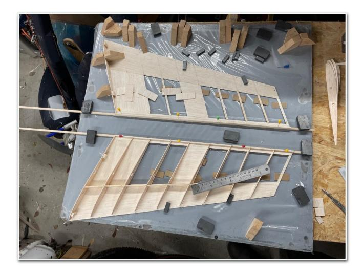
A false LE is then added before removing the wings from the board to sand them ready for the top sheeting.
