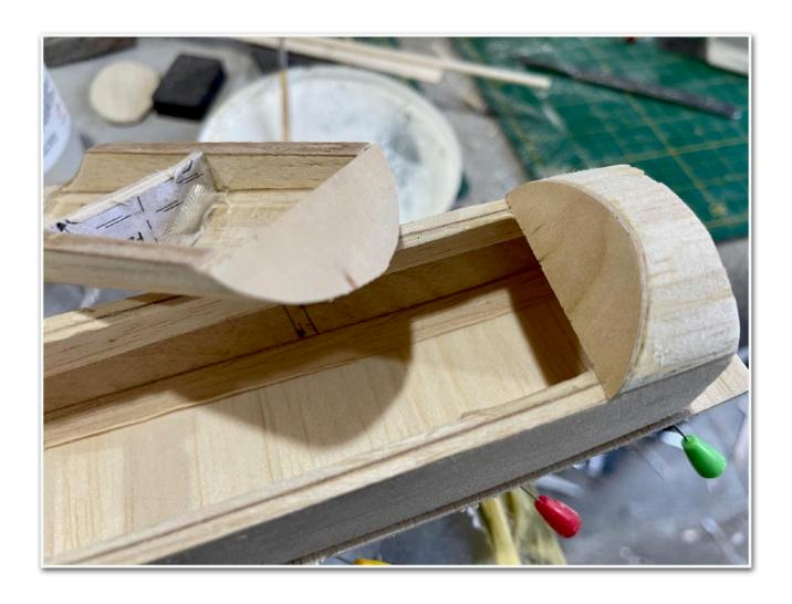
As can be seen in the previous photos, the cross grain sheeting was stuck to the bottom of the fuselage.
