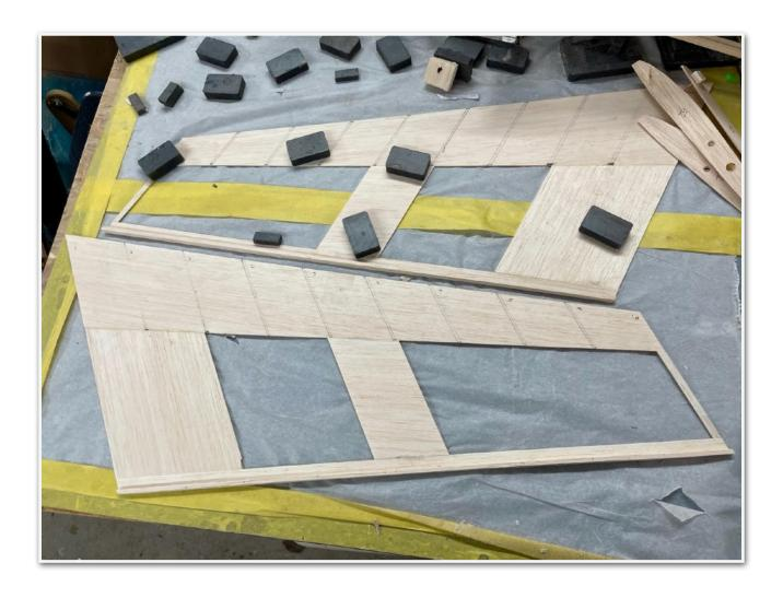
Interesting wing construction in that there are no spars. The spar webbing is, in effect, the spar but this makes for a bit of fiddly assembly as there is no spar to attach the webbing to!
