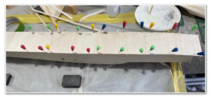
Next up was to form a ply 'crucifix' so that the balsa blocks could be attached for the nose and then sanded to shape.
