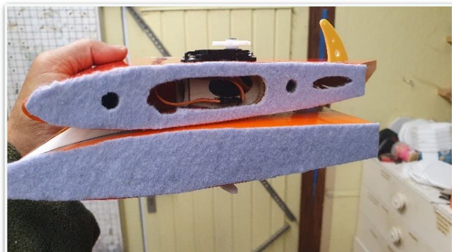
As you can see from the photo, I drew 2 lines to show the position of the carbon tube marking its depth of engagement as well. Careful application of the drill provided the connecting hole in the carbon tube and, phew, both screws worked as required!
