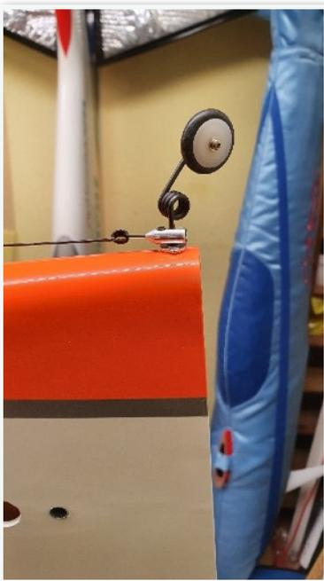
The next task was to fit the tail wheel that I had bought. It is widely used in these airframes and was relatively easy to fit. You just drill a hole, in the right place(!), and then screw the tail wheel into the fuselage. The big advantage is that if the tail wheel ever suffers damage, it is simply a matter of unscrewing the broken unit and screwing in the new one – always assuming that the manufacturer keeps on making them!
