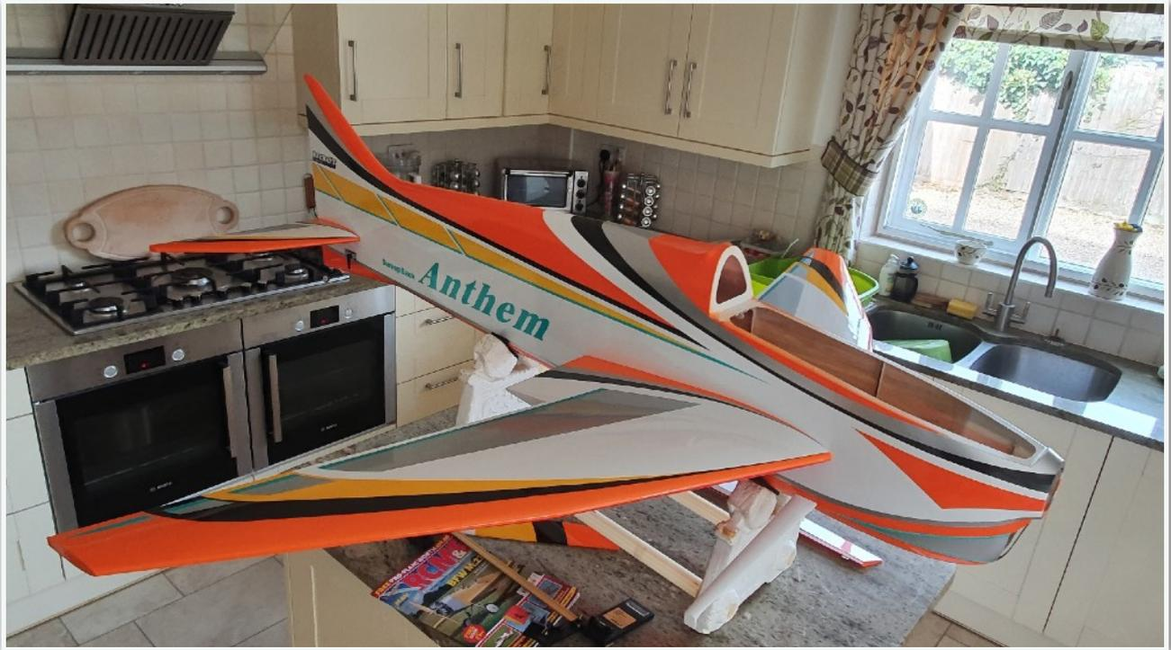
As it happened, the fixed location of the wing indicated that B J Craft had managed to get their jigs spot on as the wing incidence came out at 0.7 deg! While I was de-rigging the aircraft, I took the opportunity of checking the wing sweep and the kitchen floor tile pattern provided the ideal way to do so! It's about 18-19 deg sweep back.
