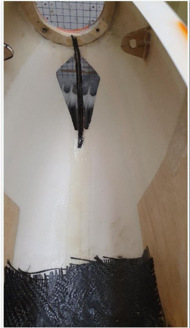
The larger photo shows the reinforcement of the rather weak structure between the 2 front air intake holes with some carbon tows. On my Agenda, which had a similar intake, the middle divider broke and so I decided to pre-empt this problem at the build stage.
