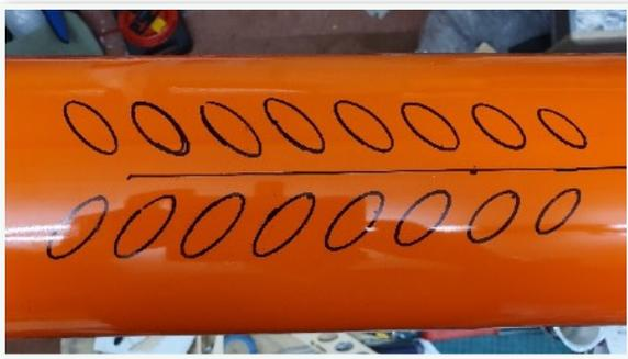
I started with the holes on the underside of the fuselage since this was flat. The photos show the initial marking and subsequent outcome. Dealing with the front intake was a bit more difficult both in transferring the pattern and in cutting out the hole!
