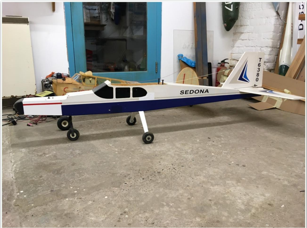
Wing, tail feathers and fuselage finished, next step is to put it all together and add weight where the engines will go to see how far forward of the leading edge they need to go to achieve balance so I don't need to add any weight.
