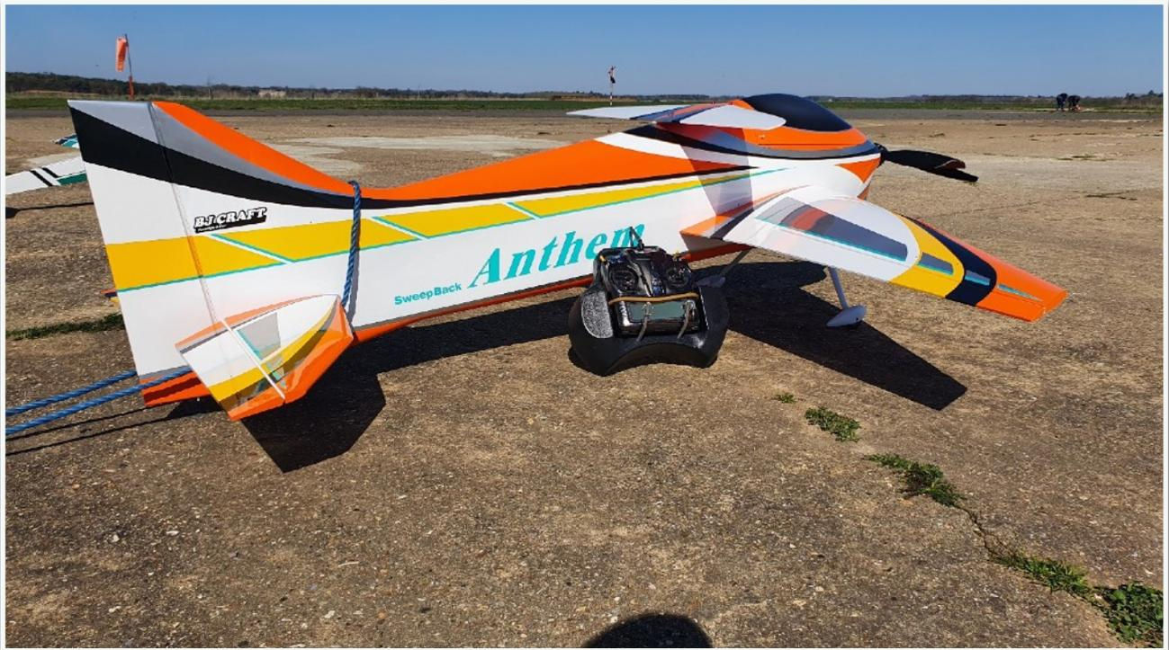
After assembling the model and checking everything over yet again, I did the obligatory range check and got a club mate to move the model through 4 quadrants to check the radio reception while doing the range check. All checked out as did the Failsafe check.
